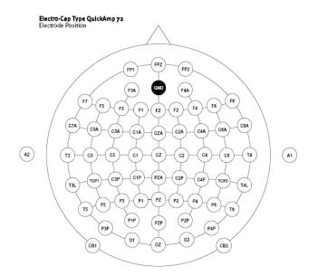
Figure 5 Electrode placement system (10/10) used in this work. The taxonomy is different than the generally used (F3A=AF3; F4A=AF4; C7A=FT7; C5A=FC5; C3A=FC3; C1A=FC1; CzA=FCz; C2A=FC2; C4A=FC4; C6A=FC6; C8A=FT8; T3L=TP7; TCP1=CP5; C3P=CP3; C1P=CP1; PzA=CPz; C2P=CP2; C4P=CP4; TCP2=CP6; T4L=CP8; T5=P7; T6=P8; CB1=PO9; P3P=PO7; P1P=PO3; PzP=POz; P2P=PO4; P4P=PO8; CB2=PO10).
